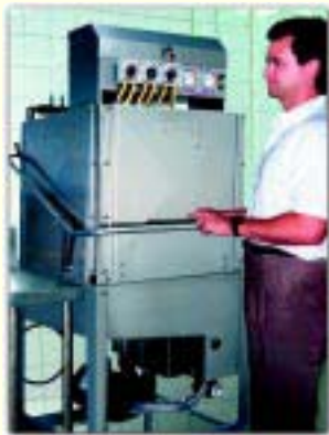
Select High or LowTemp Setting by flipping the Selector Switch on the front of the machine
