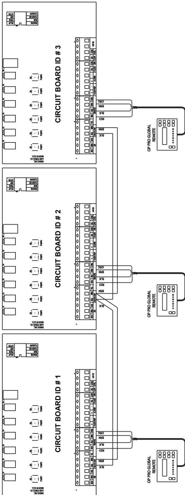
**NOTE: THIS PROCEDURE SHOULD BE DONE ONLY AFTER UNITS ARE PROGRAMMED INDIVIDUALLY WITH THREE SEPARATE ID NUMBERS AND MAKE CERTAIN THAT POWER IS OFF ON ALL THREE DISPENSERS WHEN MULTILINKING!**
