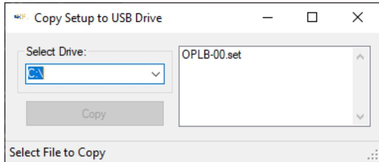
Select the USB flash drive in the Select Drive pull-down. Select the file to copy then click on the Copy button. Repeat for any other setup files.
